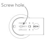
Rotate the camera clockwise to install it.
