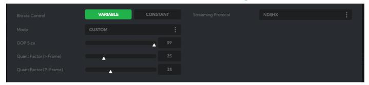
The engine encodes the camera signal into high efficiency H.264 which is then transported via either the RTMP, RTSP, SRT or NDI|HX streaming protocols.
