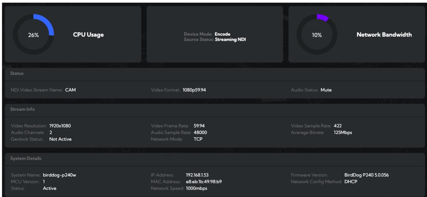
BirdDog cameras have a web interface (BirdUI) that is displayed by your computer browser and can be used to configure your camera remotely.
