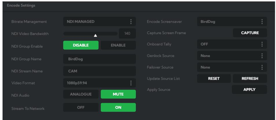
If you do opt for Manual management, you may select a bitrate within a range of 60–360 Mbps. Do this with care, as the actual bitrate may be greater, straining the capacity of the network and the receiving device, and lower settings may result in reduced image quality.
